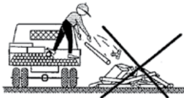
Incorrect way to off-load
